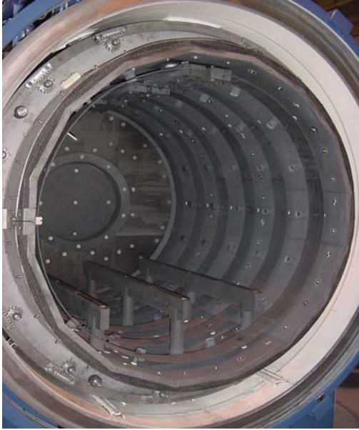
Photo. 4 Seco/Warwick 2.OVPT-4050/48HV vacuum furnace with a graphite heating chamber.
