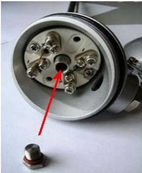
Photo. 2 Dual "S" type thermocouple (Controlling and Over-Temperature) adapted to the requirements of SAT inspection procedure in compliance with AMS2750D.
